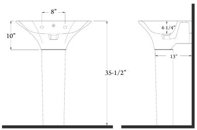
Dimensions of fixture are nominal and may vary within the range of tolerances established by ASME Standard A112.19.2-18. Dimensions and specifications subject to change without notice.
